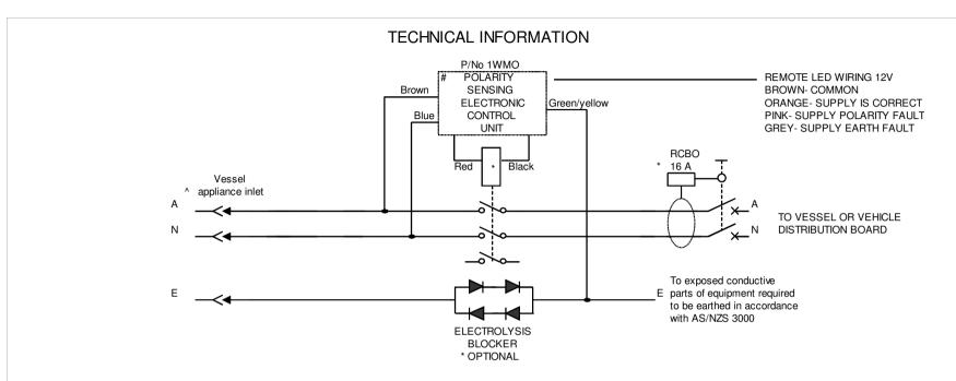
The polarity sensor is manufactured and complies with AS/NZS 3100:2002 The polarity sensor can be applied under the AS3004.2: 2008 S5.5.3.2 a,c. (Protection against reversal of polarity in the supply lead) and NSCV Part C Section 5 Subsection 5B (Electrical) Paragraph 4.7.1.c (Shore Supply).
